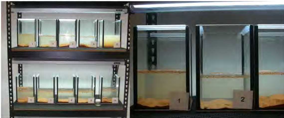
Plate 2.4 – Aquarium Set-up for Processing Sediment Samples
