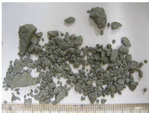
Figure 3-11: Example of siltstone intersected during drilling at CWB17 over 50-106 m depth
