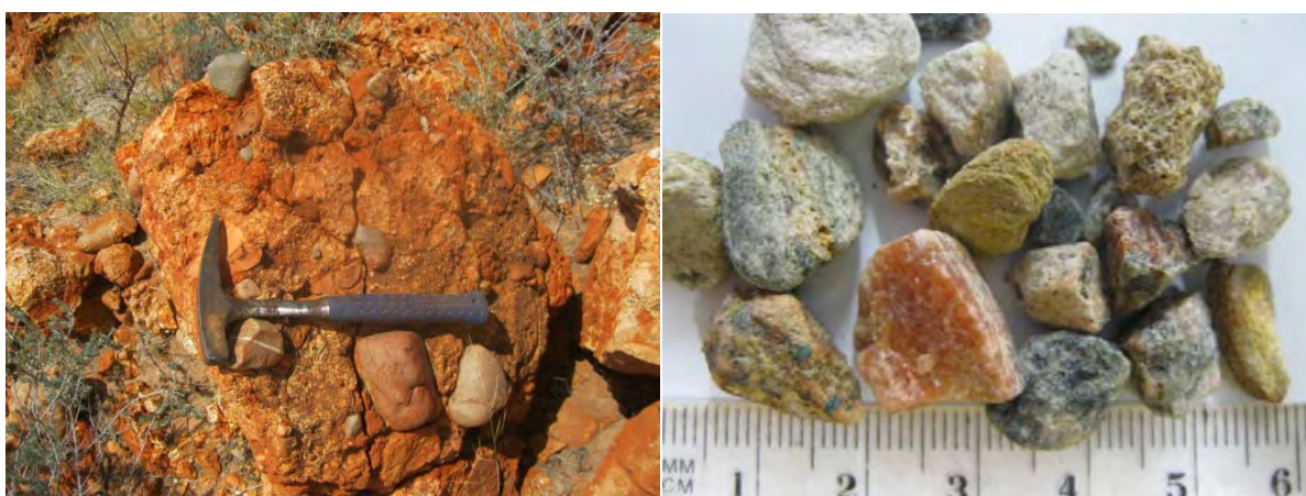
Figure 3-10: Outcropping Paterson Formation 7 km north of Kintyre, and polymictic paraconglomerate intersected in hole CWB17 at 28–42 m
