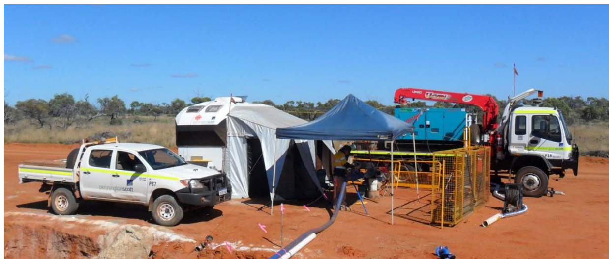
Figure 3-1: Hydraulic pump testing being undertaken on a bore at Kintyre
